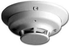
Smoke detectors are part of the fire alarm system and are typically installed in common hallways and at the top of the exit stairs. When smoke is detected, the smoke detector will activate the fire alarm system, sound the bells and send a signal to the Fire Department through the monitoring station.
