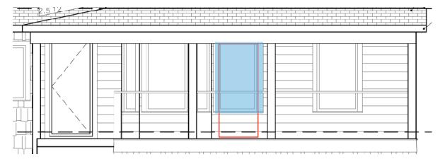
Remove existing door (outlined in red) and partially enclose the opening to convert it into a window opening (light blue), matching the size and style of the other windows on the facade. Use salvaged siding removed from the rear elevation to patch up the facade wall.
