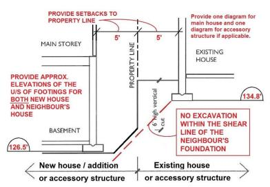
might include cross sections to show that all excavation work will have vertical cuts less than 4' deep and all other cuts will be benched no steeper than forty-five degrees.
