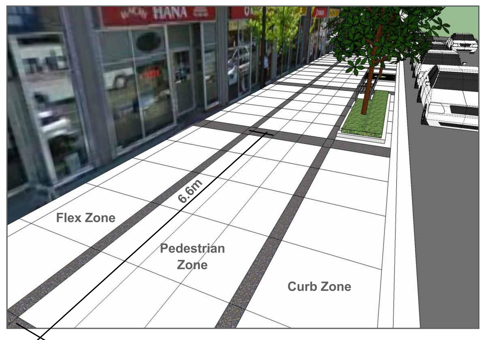
Sidewalk Field: Light, broom finish concrete Banding: Exposed aggregate
