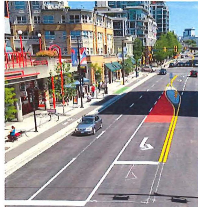
Red bus lane markings are added in at Rogers to support bus access to Lonsdale Quay.
