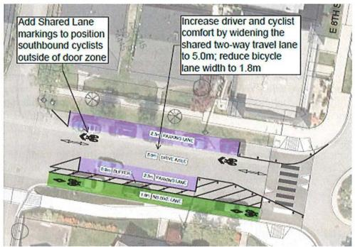
Figure 8: Roadway width adjustment
