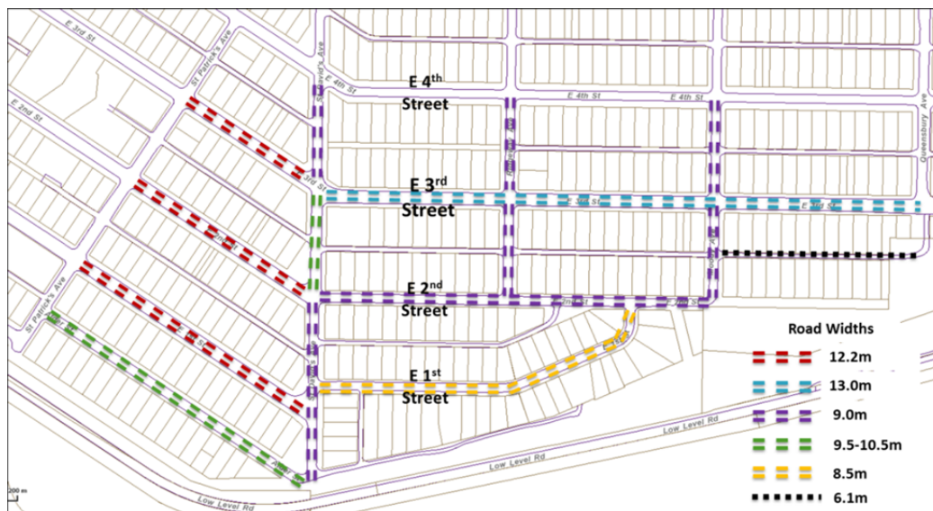
Figure 6. Road Curb-to-Curb Widths in the Moodyville Area
