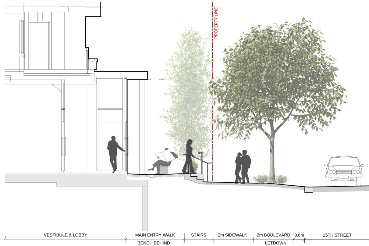
**A** SECTION - LEVEL 1 SECTION THROUGH VESTIBULE MAIN ENTRY
