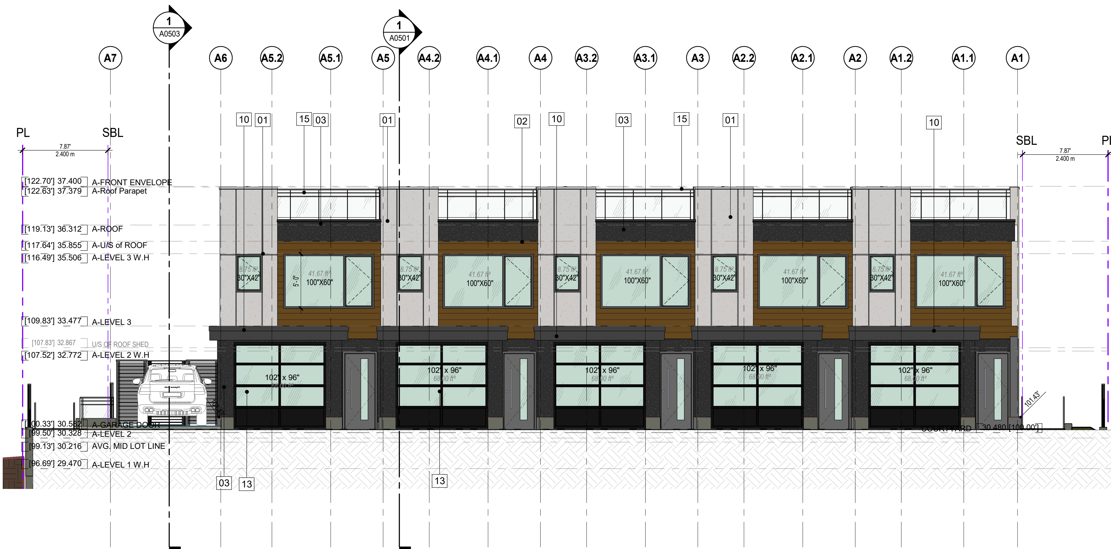
2 BLDG-A ELEVATION NORTH SCALE: 3/16" = 1'-0"
