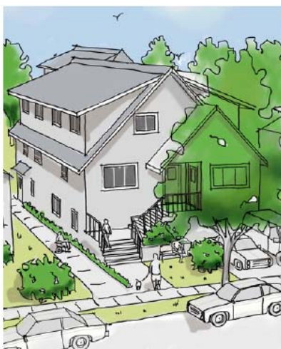
Houseplex concept sketch showing integration of front entry stairs, parking, landscaping and accessible paths of travel to rear unit
