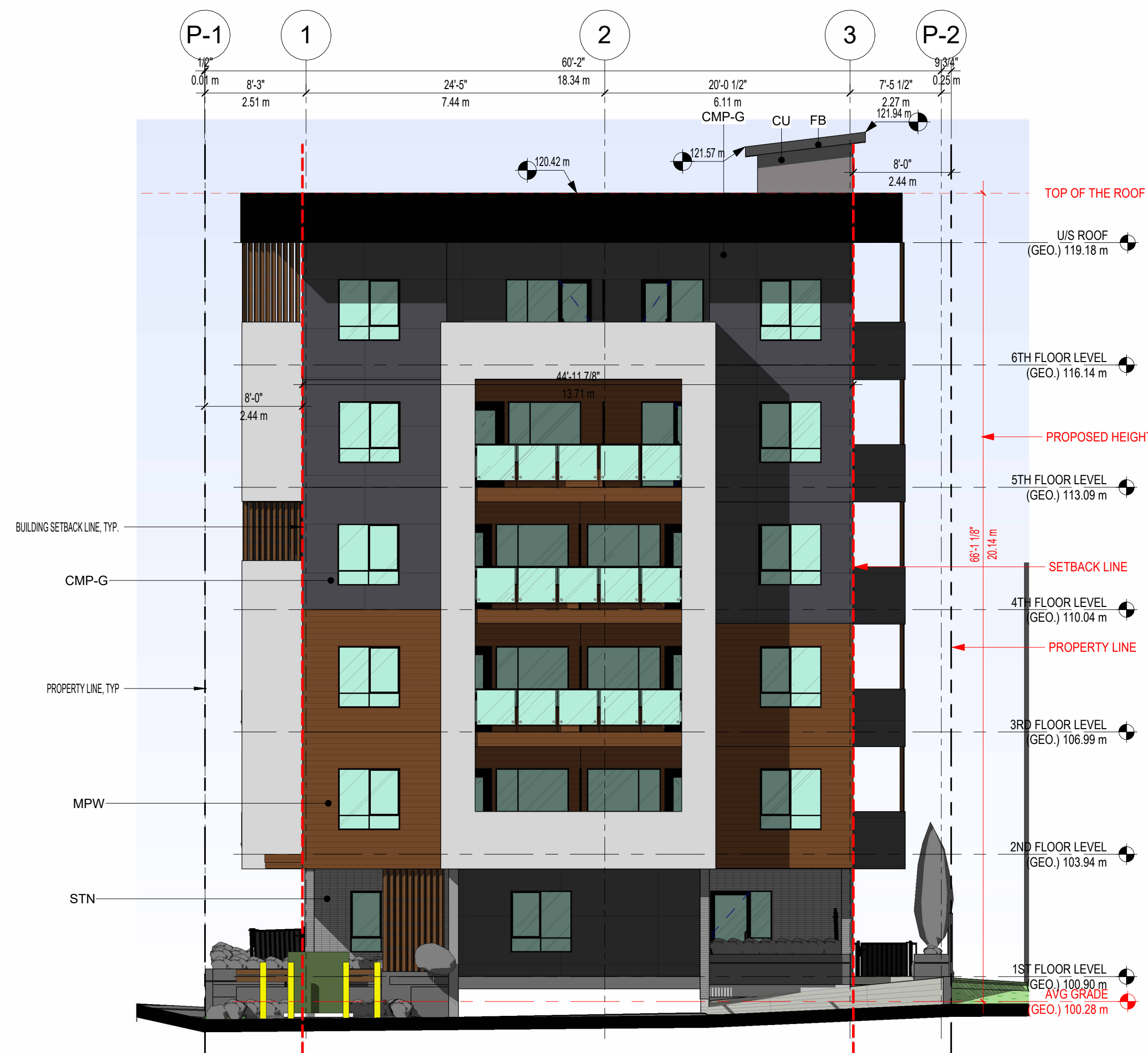
1 DP- SOUTH ELEVATION 1/8" = 1'-0"
