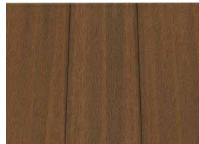
2. HORIZONTAL 6" SHIPLAP SIDING NEWTECHWOOD OR SIMILAR PERUVIAN TEAK
