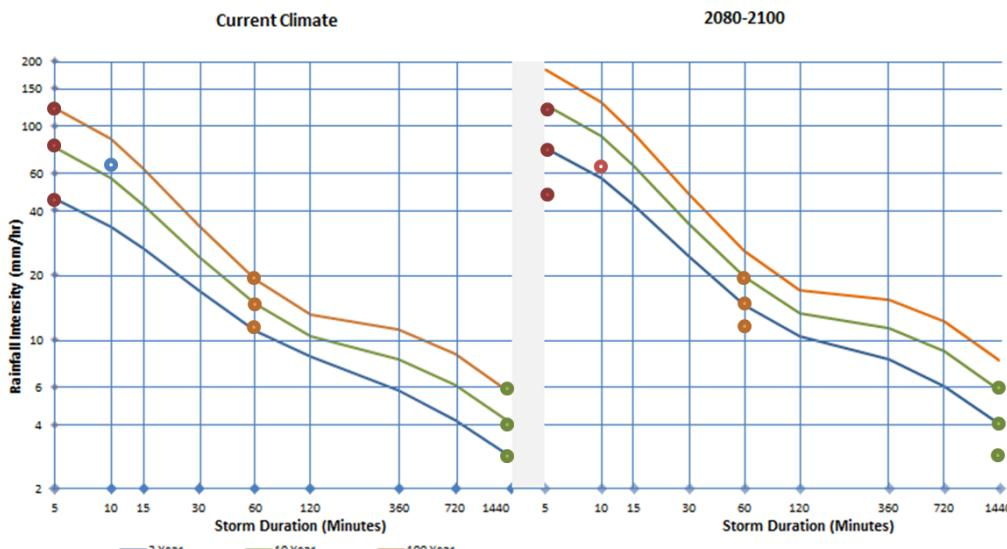
**Figure 2-2: Estimate of Short Duration Storms For RCP 8.5 Scenario**
