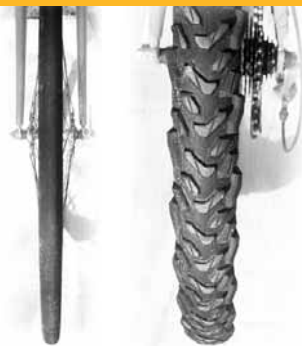
Narrow tires (left) inflated to higher pressure provide less rolling resistance, and therefore easier pedalling, on hard surfaces, while fat tires (right) provide more comfort and better traction, especially if riding off-road. Ask your bike shop what type of tire would be best suited to your riding needs.
