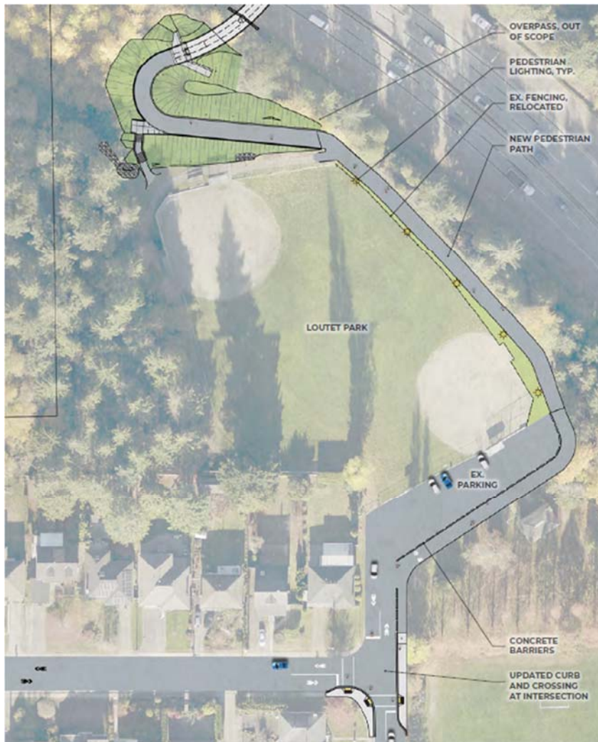
Figure 4: Intersection and pathway improvements to connect the mobility and sidewalk network to the new Casano-Loutet Overpass. The pathway will include the installation of new pedestrian scale lights to improve comfort and safety after dark.
