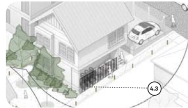
Garbage and recycling are screened from view. In this case, it is combined with bike storage.
