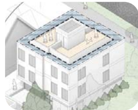
Limit the flat plane of the usable rooftop space and offset it from the building's edge.
