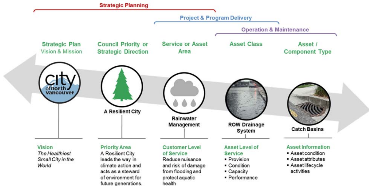
Figure 3: Service delivery line of sight (adopted from Region of Peel's Enterprise Asset Management Plan)
