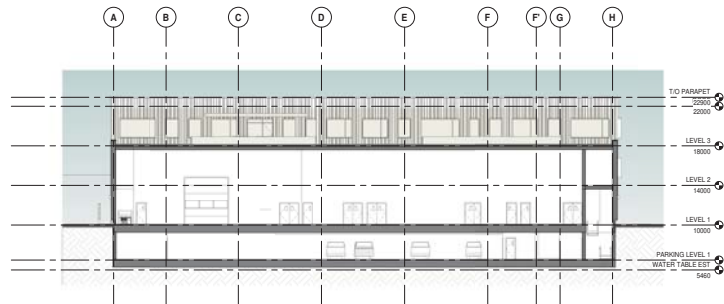
Section 3 A-106 1 : 200 ALL BUILDING HEIGHTS TO BE CONFIRMED ONCE STRUCTURAL SYSTEM IS CHOSEN
