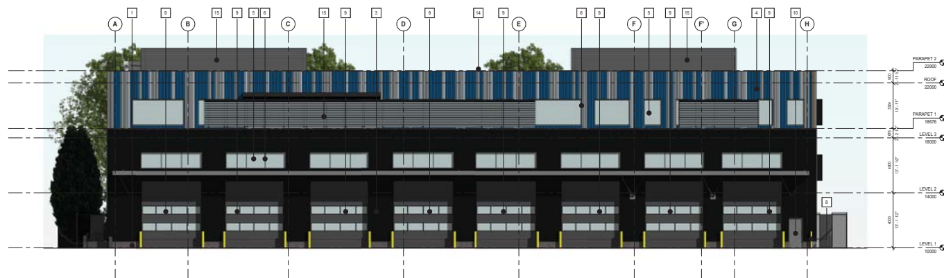
2 MAIN BUILDING - WEST ELEVATION SCALE: 1:100
