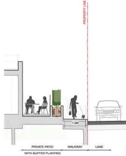
C SECTION - LEVEL 1 AT LANE Scale: 1:50
