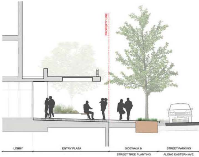
A SECTION - LEVEL 1 MAIN ENTRY Scale: 1:50
