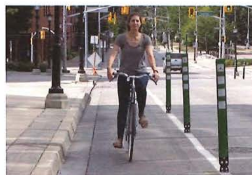
Water Street, Kitchener: Delineators used to create separation between users
