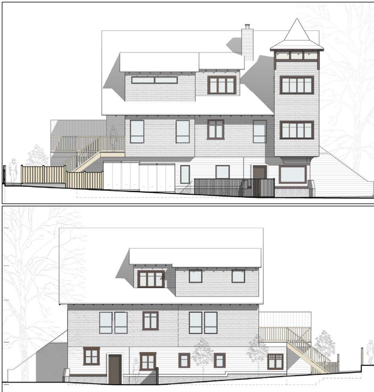
Figs. 17a and 17b: Top (Fig. 17a) shows the western side view of the Knowles Residence at 328 W 14th Street, 2021, and the bottom (Fig. 17b) shows the eastern side view. Note that the brown windows with the thicker casings are the heritage windows that will be preserved either in-situ (as is the case with those illustrated in 17a), or with those repurposed from the back elevation to along the eastern side (as is the case with some of the windows illustrated in 17b). Any new windows introduced on the building are distinguishable as new, but are compatible in design being the inverse of the heritage windows. (Source: METRIC Architecture)
