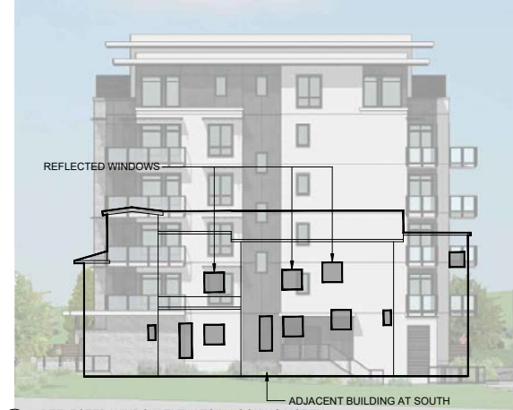
5 REFLECTED WINDOW ELEVATION LOOKING NORTH SCALE: 3/32" = 1'-0"
