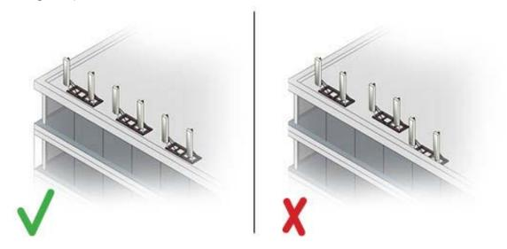
Figure 1 Antenna alignment
