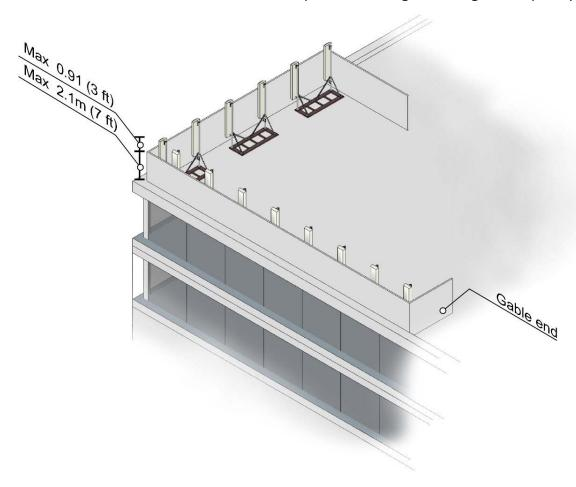
Figure 2 Screening structure
