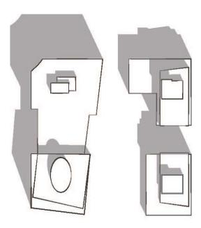
Figure 3. Sun shade diagrams can help determine the siting of buildings to minimize overshadowing of adjacent open spaces and buildings
