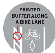
**Painted Buffer:** A painted **Buffer** along a bike lane increases the gap between vehicles and cyclists. Cars should not travel in or park in a painted buffer.
