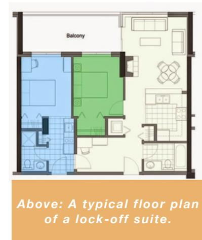
*Above: A typical floor plan of a lock-off suite.*
