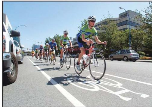
**FIGURE 2: Major street with wide curb lanes and "sharrow" markings (with room for bikes to ride side-by-side with vehicles)**
