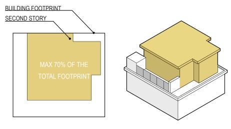
MASSING TWO STORY COACH HOUSE WITH A FLAT ROOF Image 6: Max Floor Area of Second Floor
