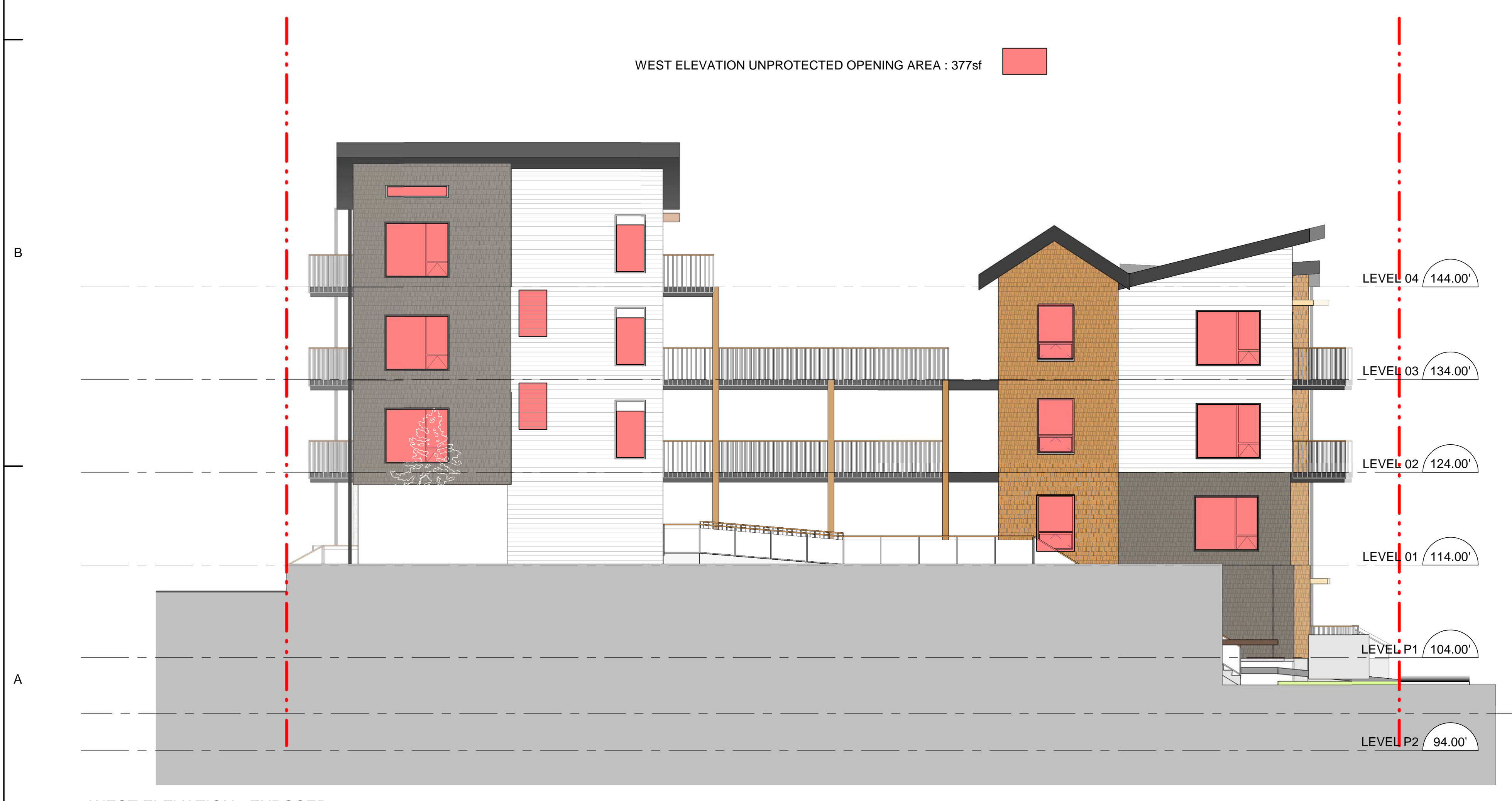
3 WEST ELEVATION - EXPOSED OPENINGS SCALE: 1/8" = 1'-0"
