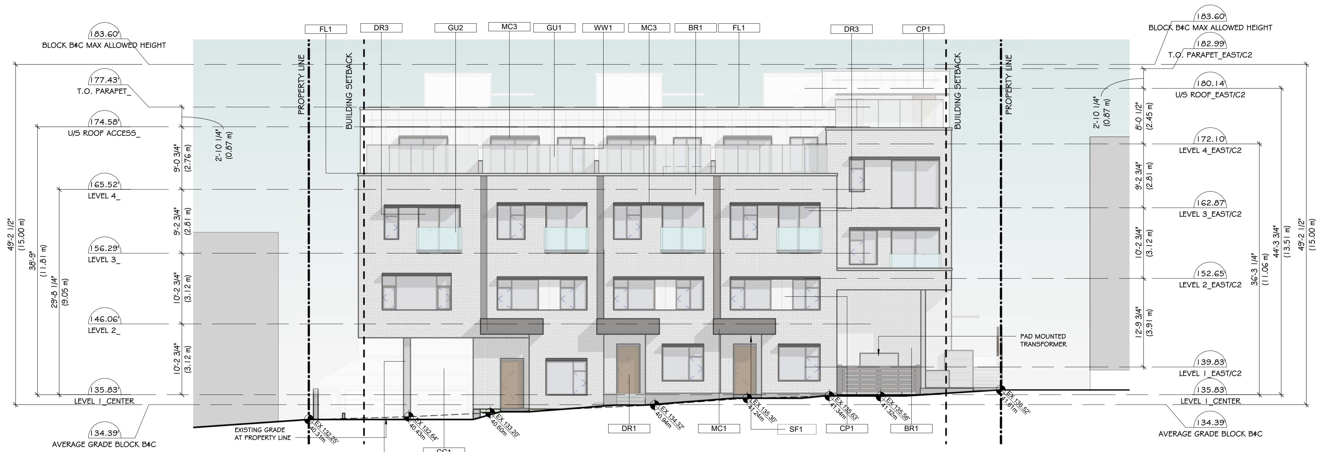
1 BLOCK B & C - SOUTH ELEVATION/ LANE 1/8" = 1'-0"
