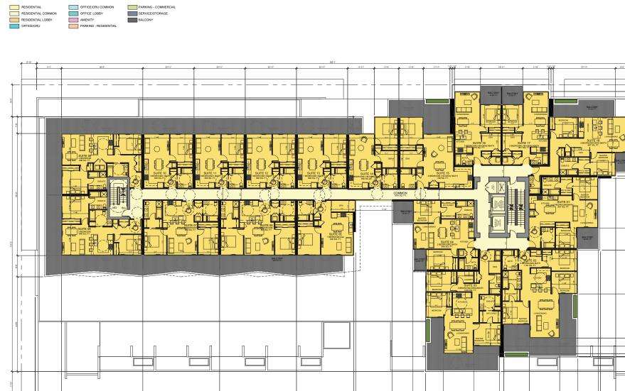
NOTE: SUITES 01,02,03,05,06,07,08,09,10,11,12,13,14 ON THIS LEVEL REFLECT REQUIRED LEVEL 2 ADAPTABLE DESIGN ELEMENTS.
