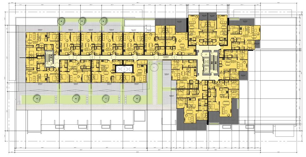
NOTE: SUITES 01,02,03,07,08,09,10,11,12,13,14 ON THIS LEVEL REFLECT REQUIRED LEVEL 2 ADAPTABLE DESIGN ELEMENTS.
