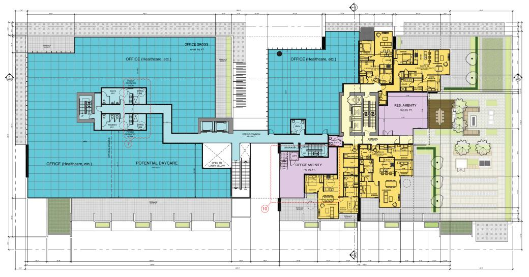
NOTE: SUITES 01,02,03 ON THIS LEVEL REFLECT REQUIRED LEVEL 2 ADAPTABLE DESIGN ELEMENTS.
